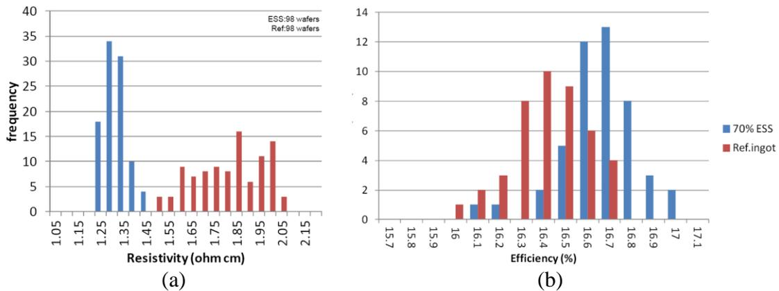
Figure 3: (a) Measured resistivity distribution on ESS wafers and poly ref wafers, (b) efficiency distribution.
