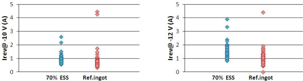
Figure 4: Reverse current measured at two different voltages.
