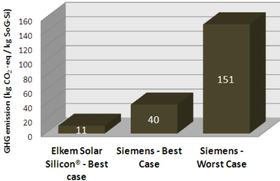
Figure 2: Preliminary results of the carbon footprint of Elkem Solar Silicon®. Comparison with Siemens production, best case with data from ecoinvent 2.2 database (with electricity and heat modified from hydropower and cogeneration) and the worst case with data from ecoinvent 2.2 database with Chinese electricity mix and heat from natural gas.
